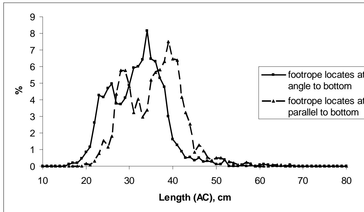
Fig. 3 Size composition of fish in catch of bottom trawl depends position of footrope
