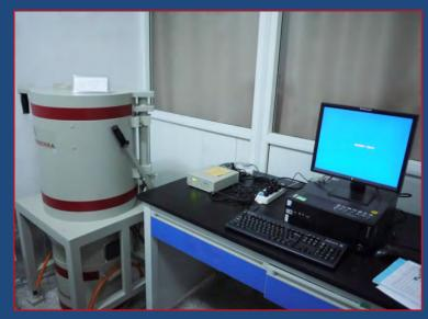
CPR HP gamma spectrometer
