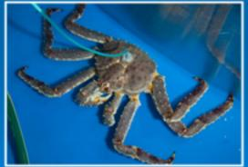
To register heart activity a miniature plastic «saddle» was glued on the crab carapace in the area of heart projection, in which it was inserted a fiberoptic sensor. Fiber has consistently joined the laser photopletizmograph, with which the signal via analog-to-digital converter enters a computer and processed with special software.
