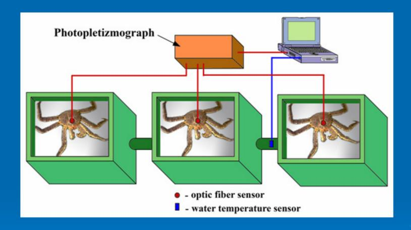
The experiments were conducted in isothermal tanks with nontransparent cover (to reduce external stress effects) of 200 and 500 liters in the artificial seawater with a temperature of 5 to 8 °C and salinity - 32 ‰.
