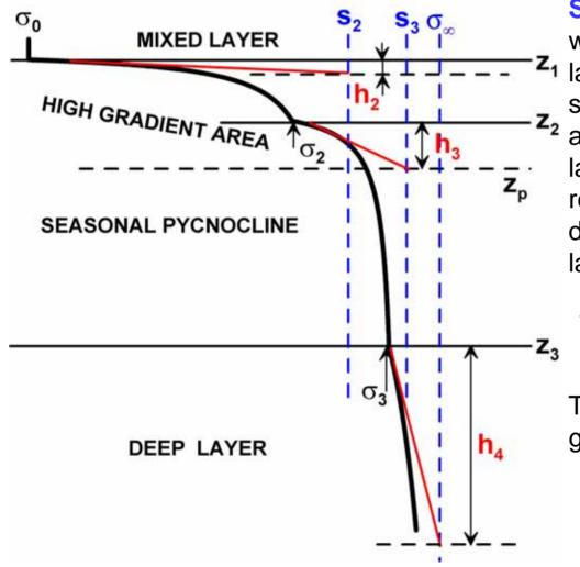
S₂, S₃ and • are the limiting values, to which sigma-t for the corresponding layer tends asymptotically. Inclined straight lines represent tangents to the approximated curve at the top of the layers. Thus, parameters h₁ are related to the maximum value of a density gradient in a corresponding layer
