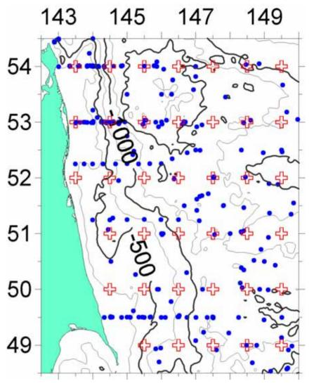
The mean density field was constructed on the 1° grid (38 nodes, +).
