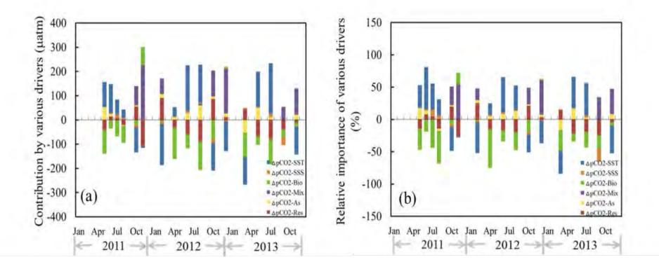
Contribution (a) and relative importance (b). (a) and (b) of various processes (temperature, salinity biological effect, vertical mixing, air–sea exchange, and a residual term) to the  $pCO_2$  at the A4HDYD station.
