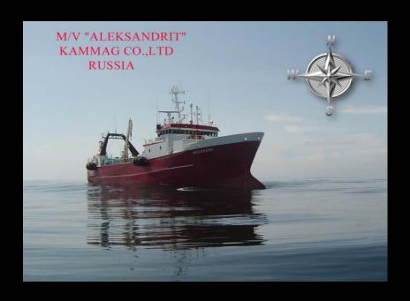
Built in 1985, length – 48.250 m, width – 11.0 m, draught – 5.5 m, power of general engine - 2250 l/sec, speed – 9 knots. The fishing gear used was shrimp bottom pair trawl «Cosmos-2005» made in Denmark. The mesh of the trawl wings is 20 mm, the opening - 35x2 m. The trawl has temperature and depth sensors and selective greed, set in not far from entrance.
